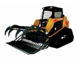
Rock Bucket and Rock Bucket with Grapple also available for skid steer loaders and tractors.
