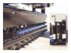
Adjustable Rhino-Hide Barrier Quickly choose the size of material you want to leave on the seedbed. Raising barrier promotes faster soil drying. The barrier is stiff for pushing yet flexible enough to allow damage debris to pass.
